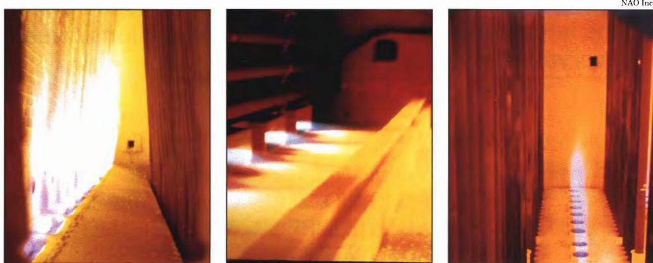
**FIGURE 1.** These burners—all combusting natural gas—are installed either vertically (for reformers) or horizontally (for cabin heaters)
